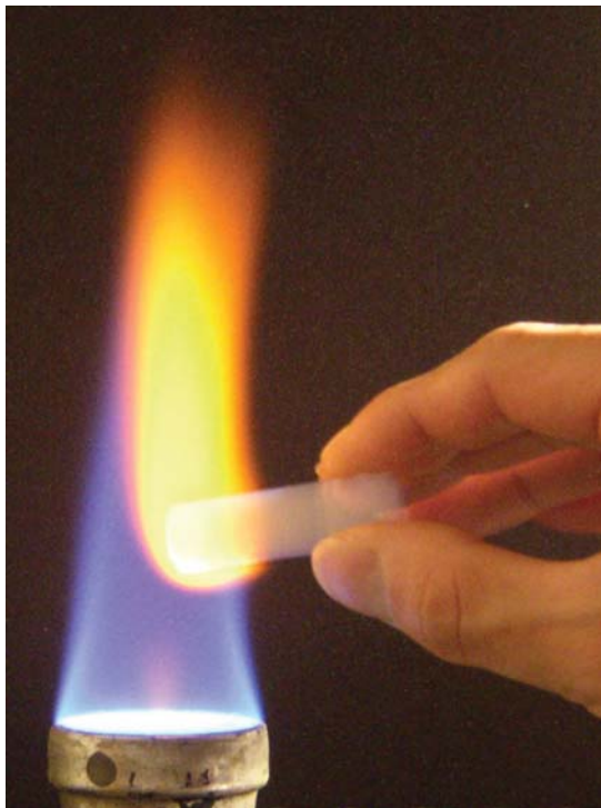
Figure 5.3 Owing to its extremely low thermal conductivity, a piece of inflammable aerogel can be held in a butane-torch flame for prolonged periods of time without burning one's fingers. In this photograph, a student has been holding the slab of aerogel for over a minute
