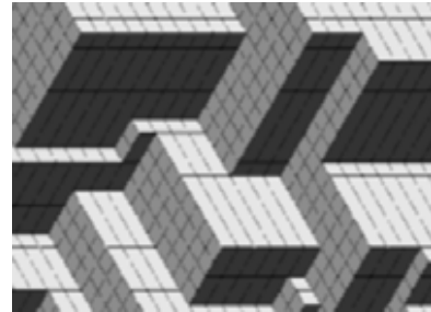
Fig. 11.10 Logarithmic growth of an interface. A simplified model of an interface perpendicular to a body diagonal in a frustrated next-neighbor Ising model with barriers to coarsening that diverge with length [132]. Notice that the interface is lowering its energy by poking out into facets along the cubic directions (a kind of facet coarsening). This process gets much slower as the faces get longer, because the energy barrier needed to flip a face grows linearly with its length. This slow-down happens below the corner rounding transition described in the caption to Fig. 11.6.
