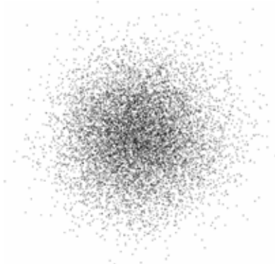
Fig. 2.6 Many random walks. 10 000 endpoints of random walks, each 1000 steps long. Notice that after 1000 steps, the distribution of endpoints looks quite Gaussian. Indeed after about five steps the distribution is extraordinarily close to Gaussian, except far in the tails.
