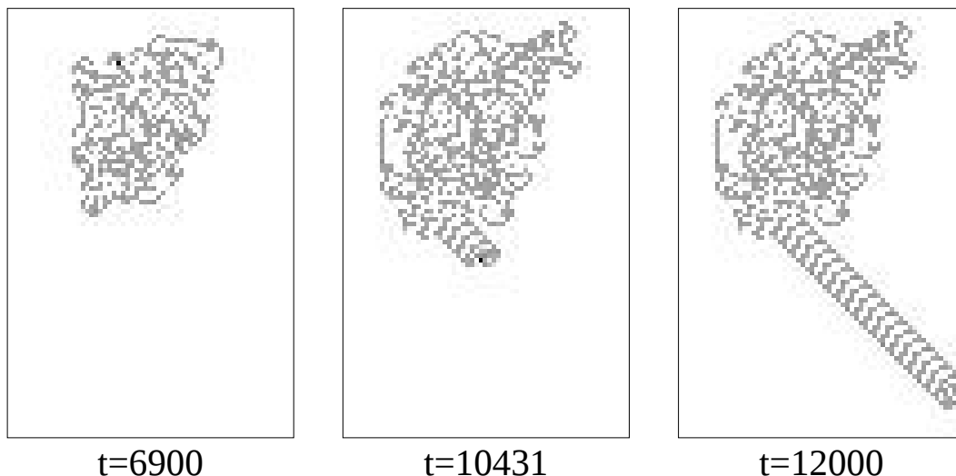
Figure 18: The Langton's ant rule. The motion of a single ant starts with a chaotic phase of about 10000 time steps, followed by the formation of a highway. The figure shows the state of each lattice cell (gray or white) and the ant position (marked by the black dot). In the initial condition all cells are white and the ant is located in the middle of the image.
