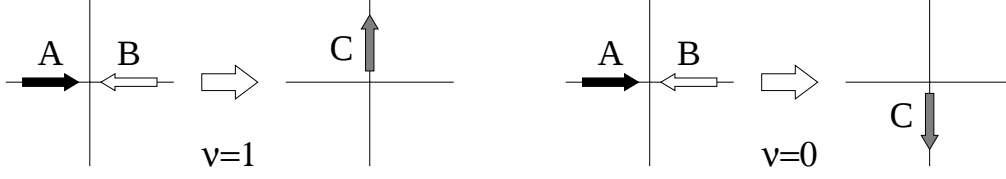
Figure 41: Automata implementation of the A + B \rightarrow C reaction process.
