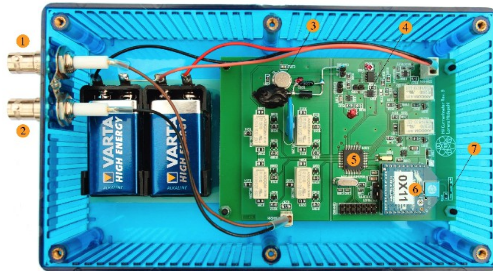
Figure 3.5: High-voltage (HV) current meter with wireless readout (open lid). (1) HV in; (2) HV out; (3) non-inverting operational amplifier (AD549L); (4) 16-bit ADC (AD7790); (5) microcontroller (MSP430); (6) XBee ® wireless transceiver; (7) reed switch. [Hö12]
