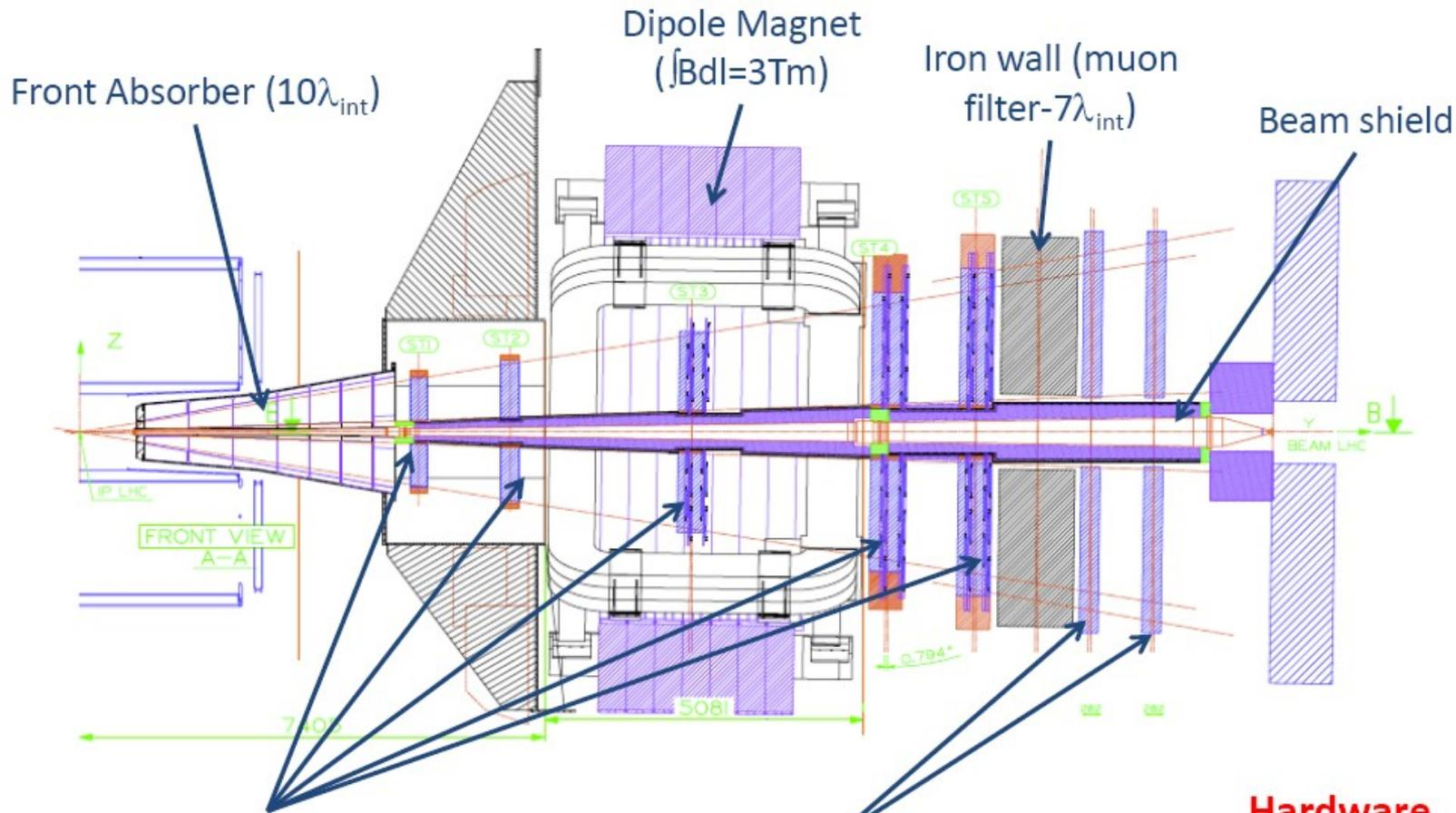
5 tracking stations (10 planes of MWPCs with bi-cathode pad readout): resolution  $\cong 70\mu\text{m}$  in the bending plane
