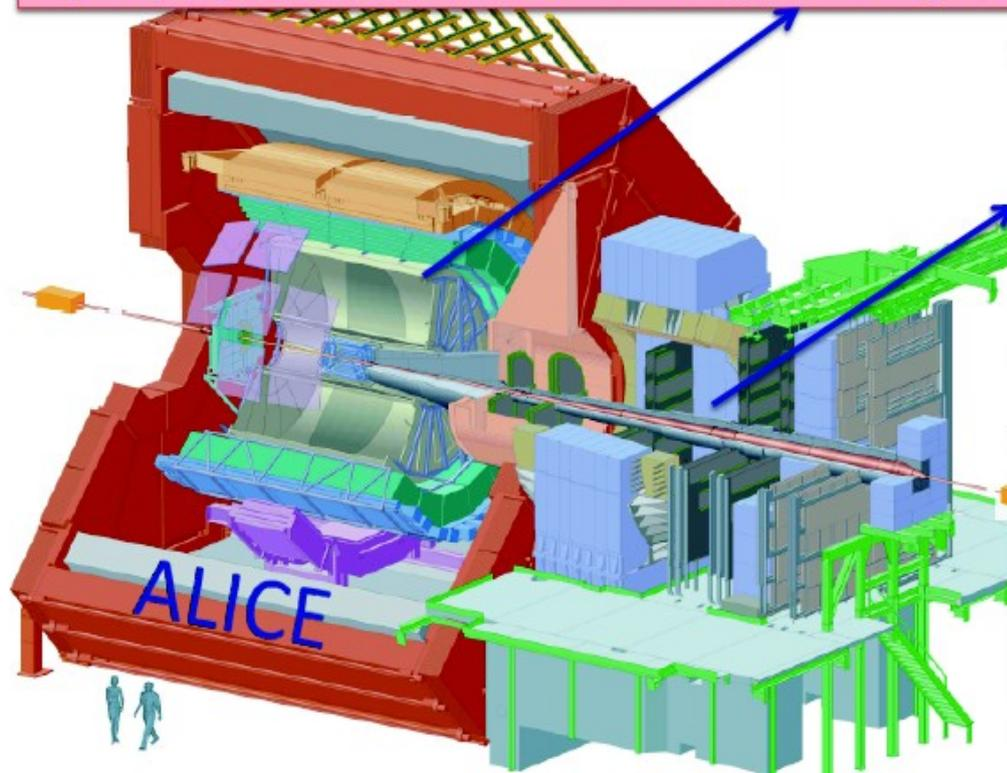
Forward muon spectrometer
