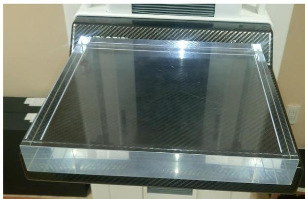
Figura 3.10: Flat field phantom
